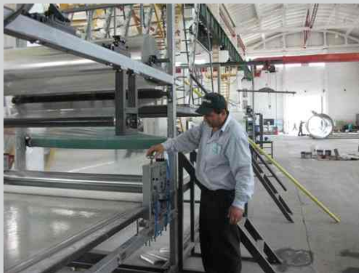
Continuous Laminating Machine Manufactured and Tested in Arkansas - USA
